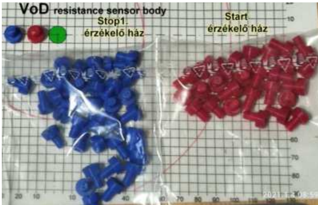
2. image Sensor probe housings for VoD measurement
