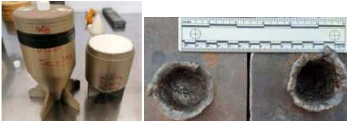
2.picture: Explosive charges and their penetration in 35mm steel without liner.
