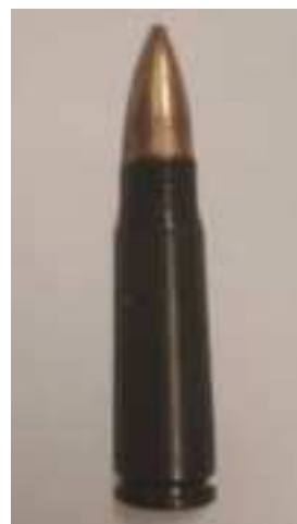
Figure 3 7,62×39 mm 43M PS steel-core projectile (Photo by the author)
