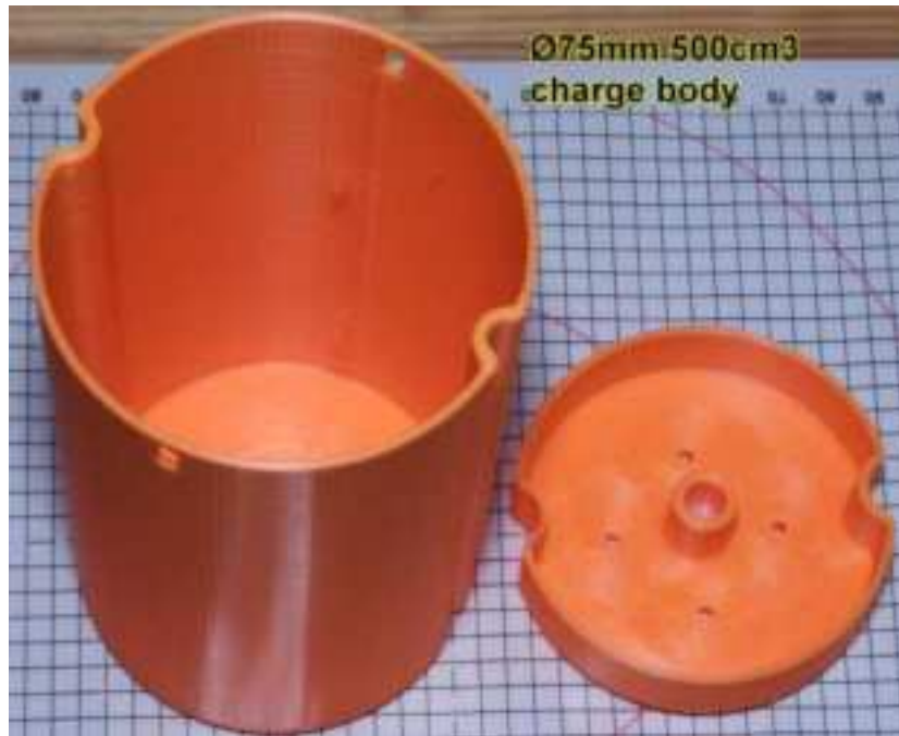
5. Multipurpose case of charge
