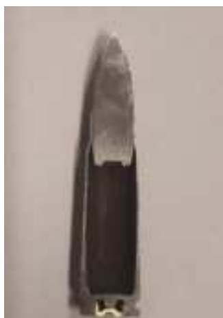
Figure 4 Section of 7,62×39 mm 43M PS steel-core projectile (Photo by the author)
