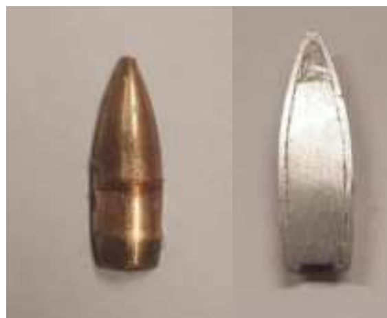
Figure 5 Section of a 43M PS projectile showing the jacket, lead ring and steel core (Image by the author)
