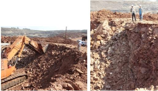
Figure 5 Shovel excavating blasted overburden (Blast #2) showing good fragmentation
