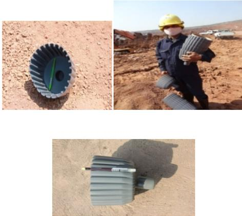
Figure 1 Stem-plugs (Vari-Stem Blasting Plugs)
