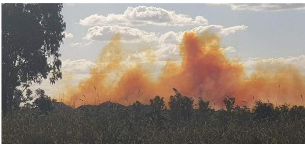
Blasting fume is hazardous. It is a combination of post blast gases, which are predominantly nitrogen dioxide and nitric oxide. Nitrogen dioxide is the visible component. Exposure to high concentrations can lead to adverse health outcomes. Authority holders have a regulatory obligation to eliminate or mitigate hazards in their operations.
