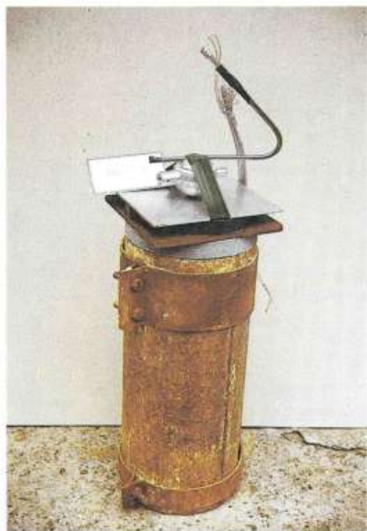
Preparation of the perforator type TALTOS-I, for performance test
