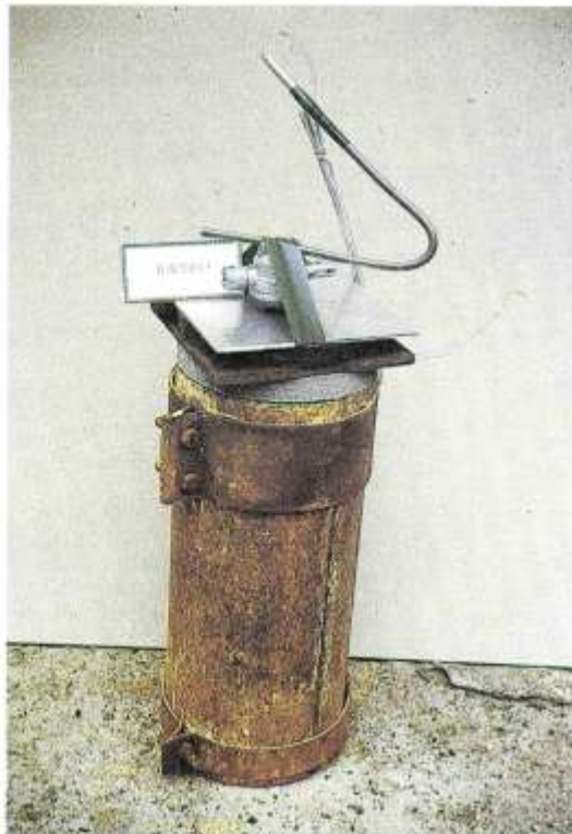
Preparation of the perforator type TORNADO JET-LINK with 2 1/8" diameter for performance test
