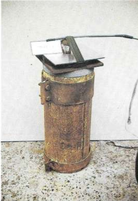
Preparation of the perforator type MIDJET-I. for performance test
