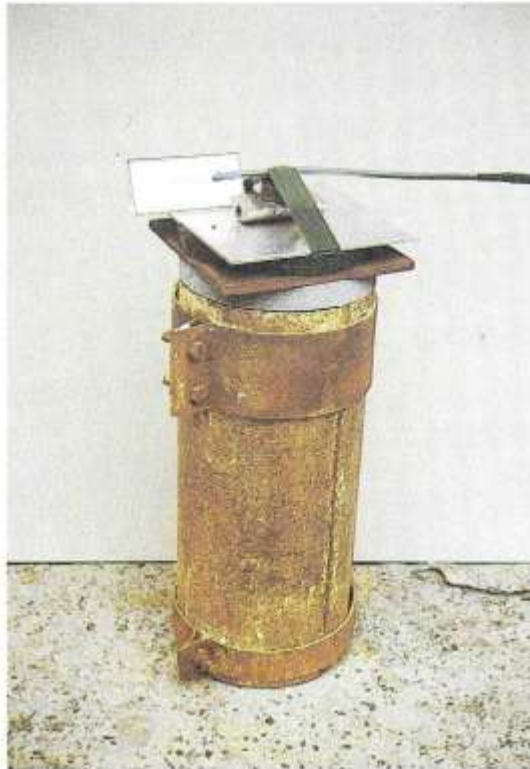
Preparation of the perforator type SMALLJET for performance test
