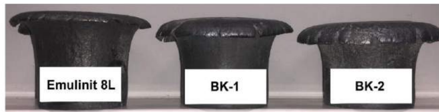
Figure 3. Comparison of brisance using the Hess test
