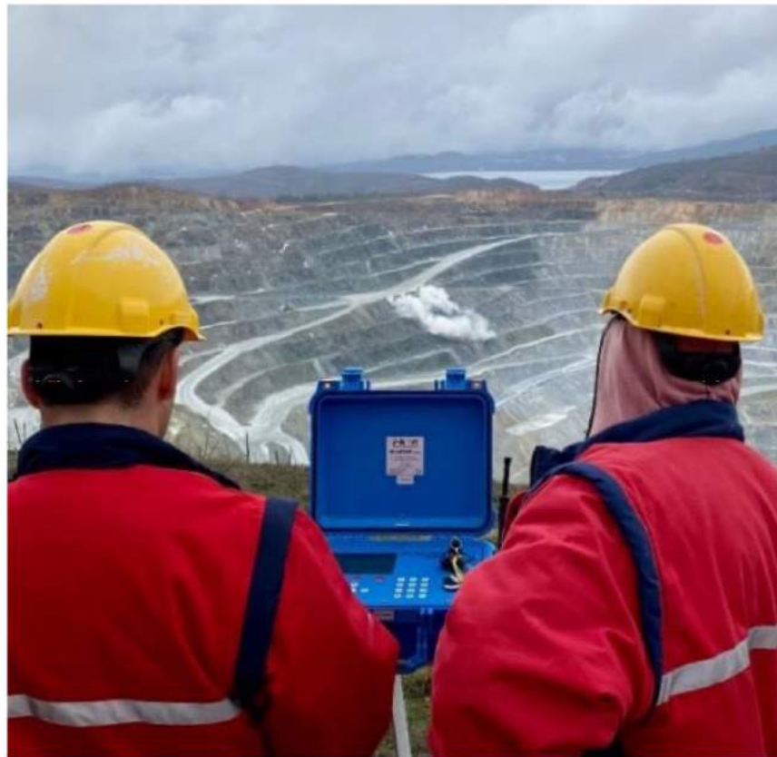
Figure 2: Mine blasters successfully and remotely firing off one blast field.
