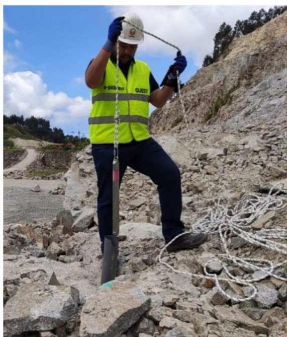
Figure 4. (left) Deployment of O-Pit DEV probe, (right) Visualization of borehole deviation on the app.
