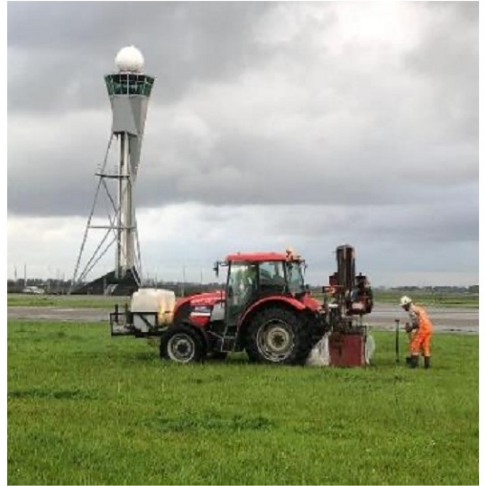
Figure 1 Sonic Drilling Rig mounted on standard agricultural tractor unit for Seismic Operations. Location Schiphol Airport, between airstrips.
