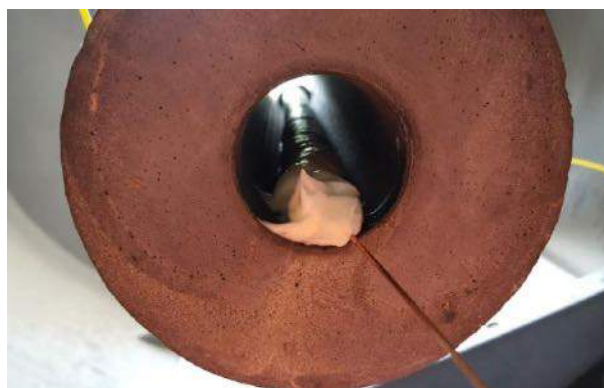
Figure 1-1: Decoupled string emulsion \varnothing 22 mm in \varnothing 50 hole and a VoD probe in a mortar confinement.
