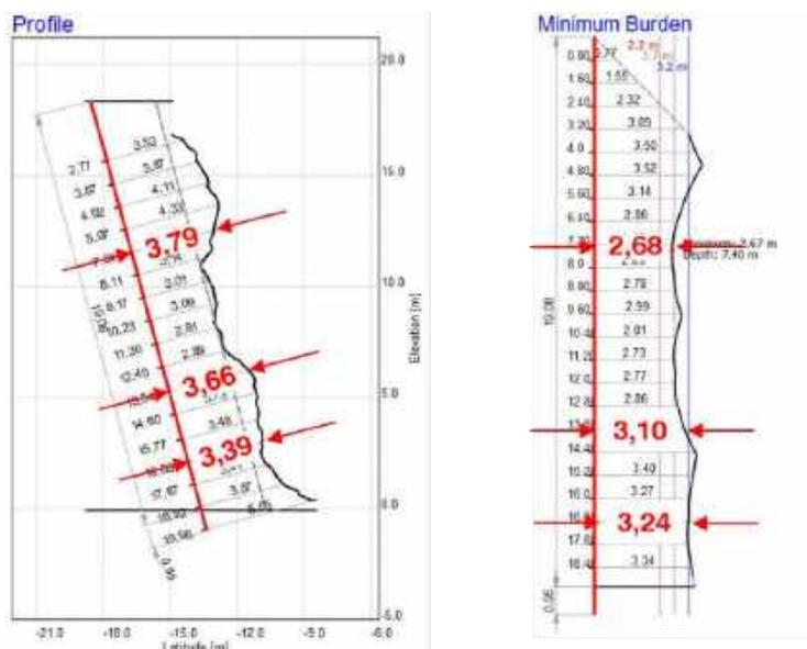
Figure 5. Profile and minimum burden diagram for the same borehole; note the significant differences at the indicated hole depths
