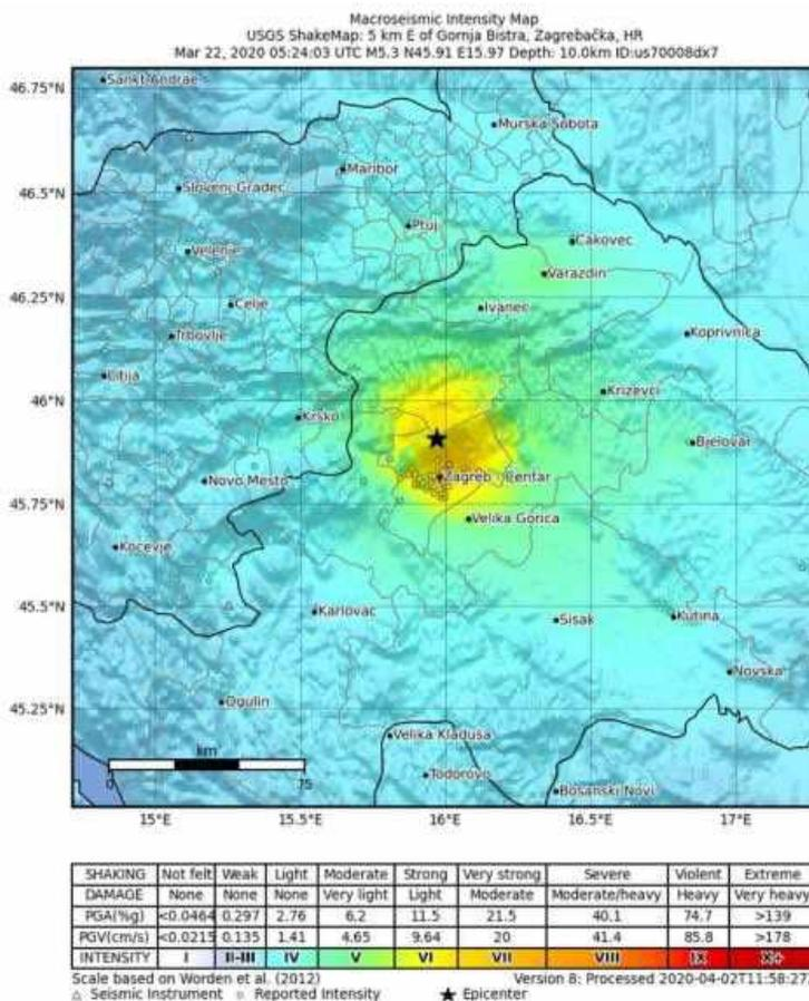
Figure 3. Epicentre and intensity of earthquake made by USGS
