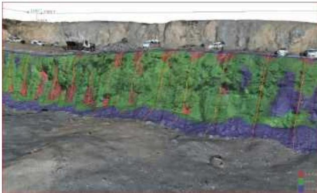
Figure 6: Minimum burden chart with indicated location of boreholes; green colour shows design burden, red: light burden, and blue: heavy burden
