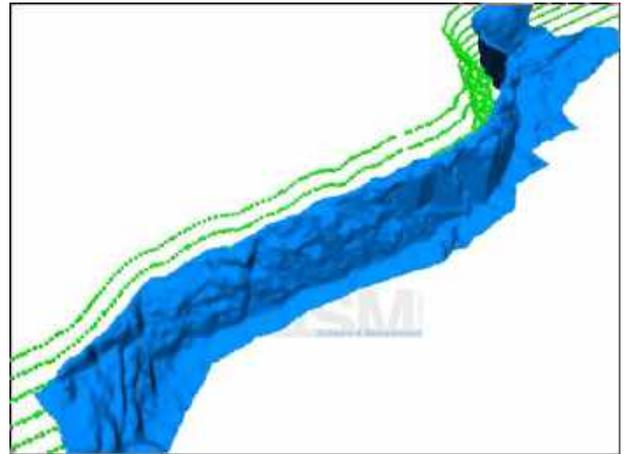
Figure 7. The computation of the minimum burden surface starts with the determination of according sample points (green)
