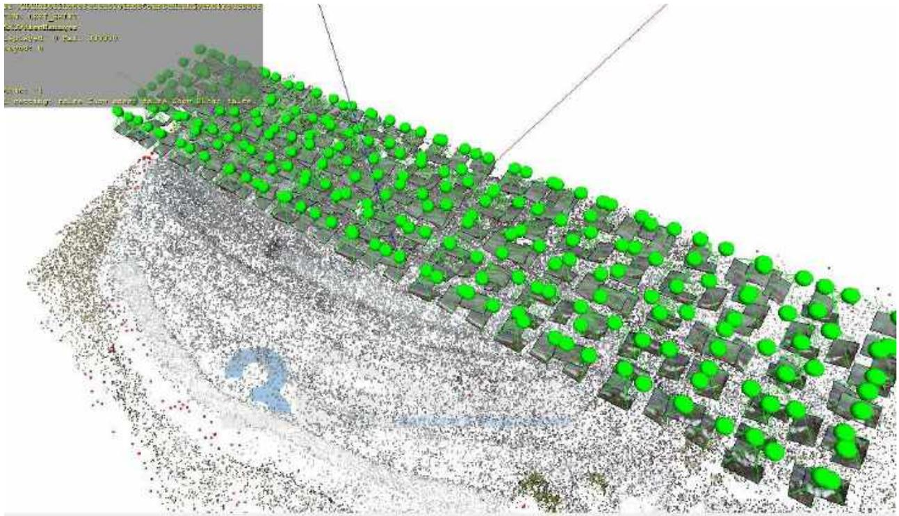
Figure 2. Analysis of deviations between camera locations from GPS recording (spheres) and photogrammetry-determined (pyramids).
