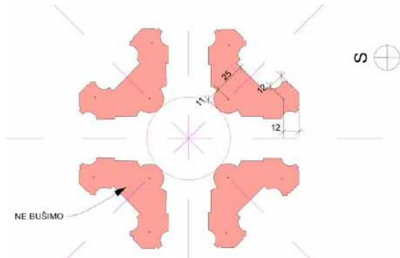
Figure 11. Positions of metal wedges
