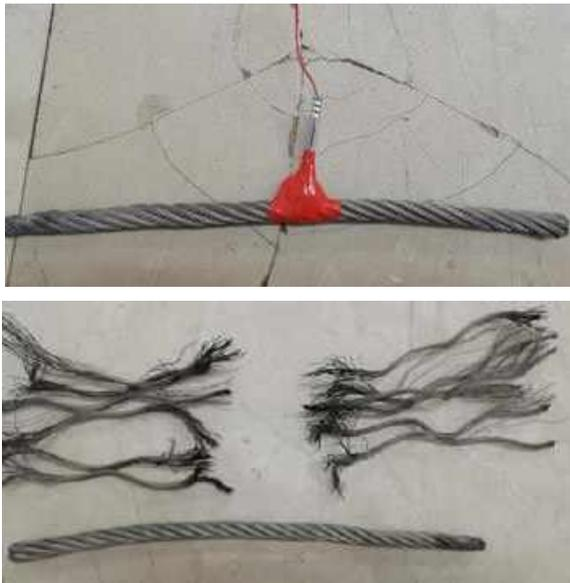
Figure 12. Wire rope explosive cutting test
