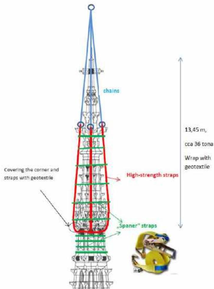
Figure 8. Preparation of northern tower for lowering by 500-tons crane [4]
