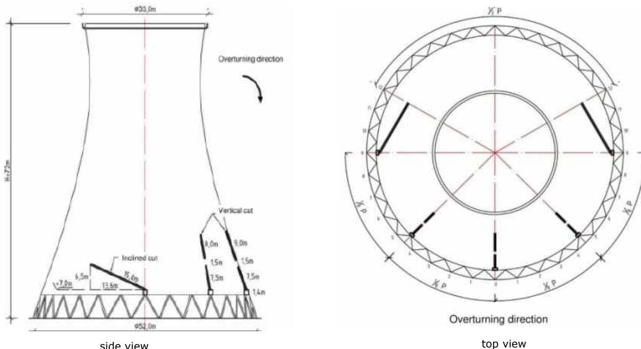
Fig. 5. Location of the cuts on tower body.
