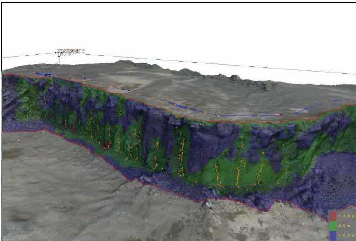
Figure 9. Minimum burden chart for automatically placed boreholes on a curved corner blast; bright dots indicate locations of minimal burden.
