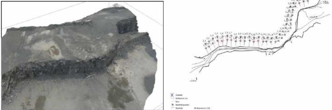
Figure 8. Left: 3D image of a curved blast site; right: plan view of automatically placed boreholes using minimum burden surfaces; the boreholes follow the crest
