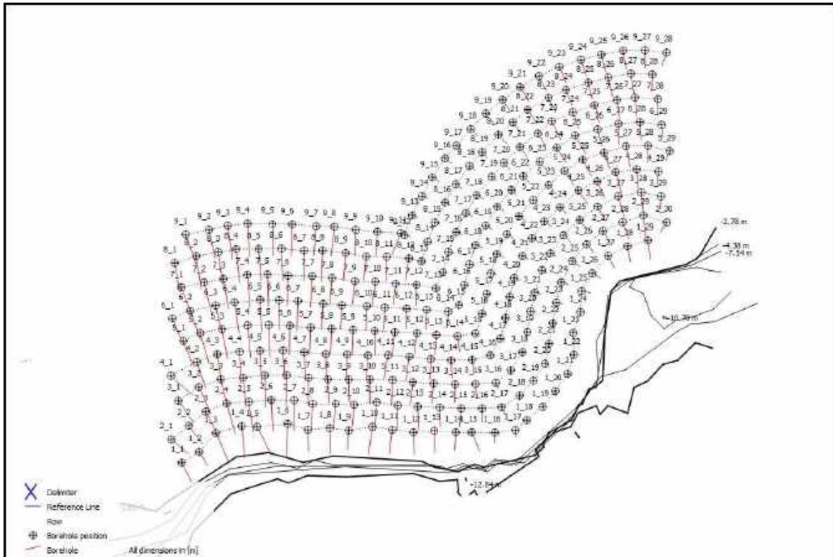
Figure 10. Automatically placed boreholes with loose constraints in azimuth and inclination
