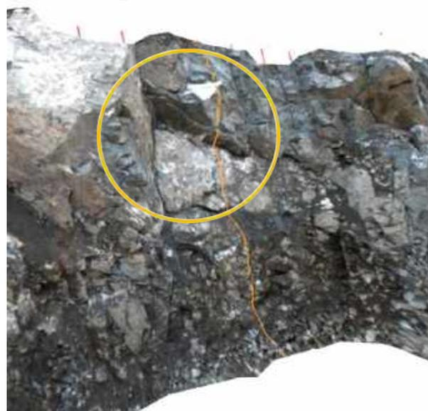
Figure 4. 3D model with a single profile; circle marks an irregularity (remainder of a detached block)
