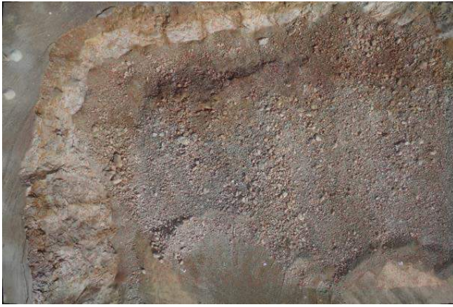
Figure 8: 3D image of a muck pile (left) and automatic particle detection based on the combination of geometric analysis and image processing (right).
