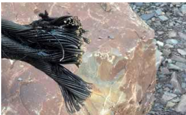
Fig. 6 b: Sample blast rope - 2. and 3. attempt: complete clean separation
