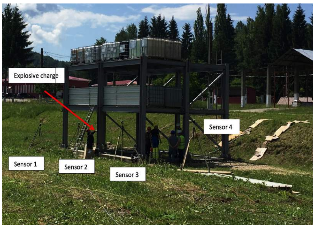
Figure 1. Overview of the steel frame specimen. a) 3D geometry, with the position of pressure sensors S1-S4; b) photo before testing
