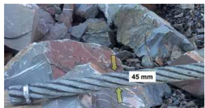
Fig. 5: Rope before sample blast
