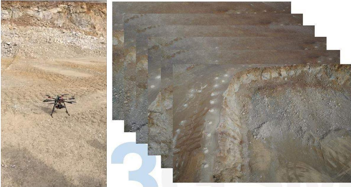
Figure 1: Drone ready for take-off in a surface mine (left) and stack of highly overlapping images (right).
