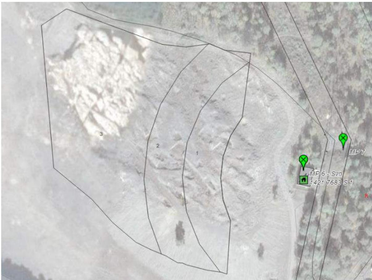
Figure 5.5. View over the zones. Excavation starts in zone 1, the zone closest to the substation (MP 6)
