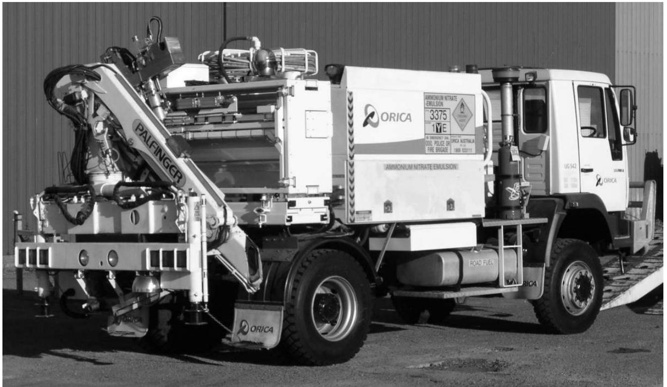
Figure 9. Early remote-control charging equipment with smart vision systems to identify blastholes
