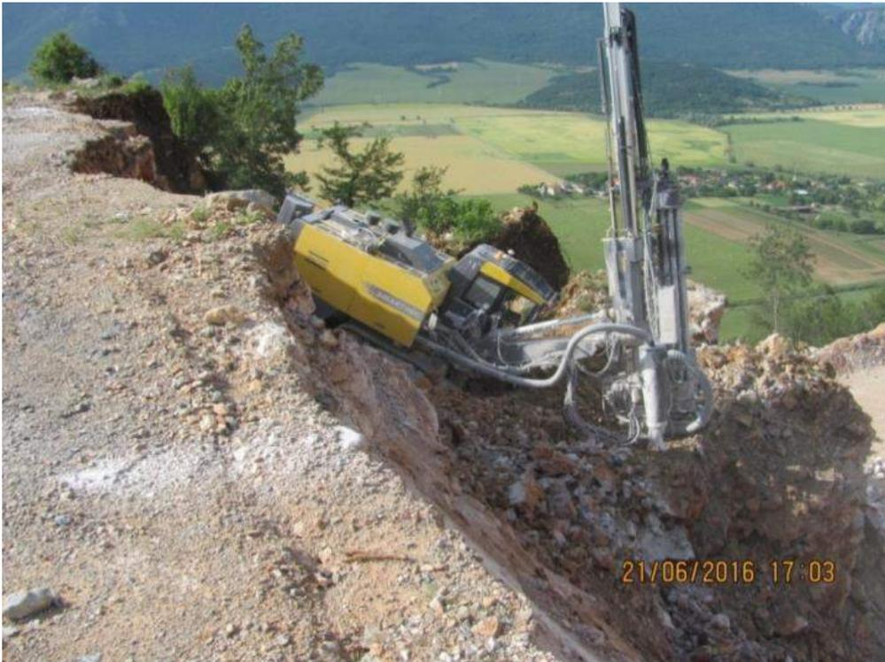
The drilling machine was approximately 5 meters below the level of the bench IV, on an inclined position, it leans on a rock and seems to be on a stabilized position.
