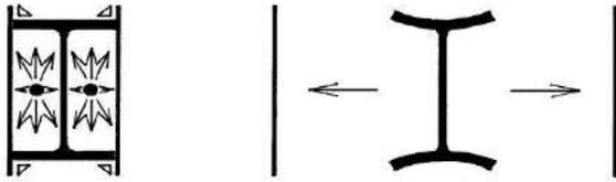
Figure 5. H-profile with plates suboptimal.
