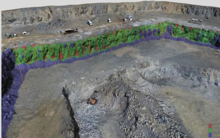
3D images from drones are a perfect survey of large blast sites. Poor blasting results are often caused by inaccuracy of the front row hole placement and suboptimal blast pattern geometry.
