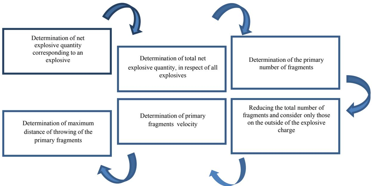
Fig.2. Process diagram for primary fragments projection
