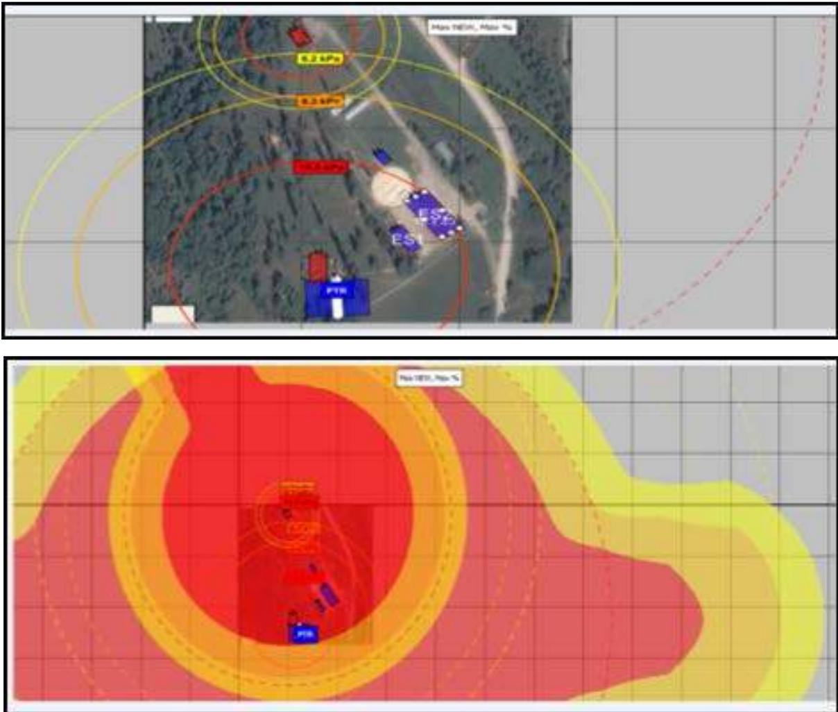
Fig. 15. Contour map for a deposit of explosives with a capacity of 1220 kg ETNT
