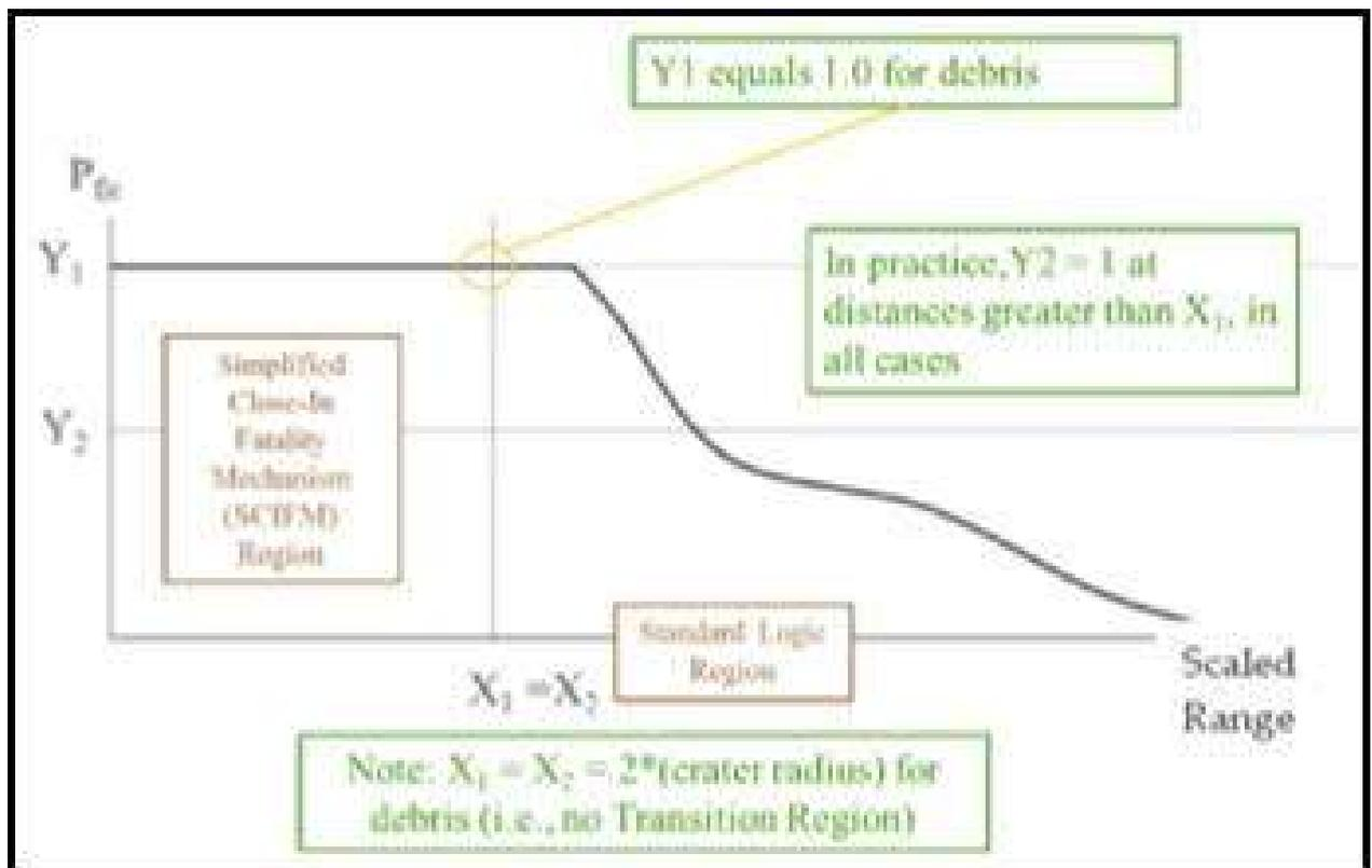
Fig. 13. The Model SCIFM for fragments projected
