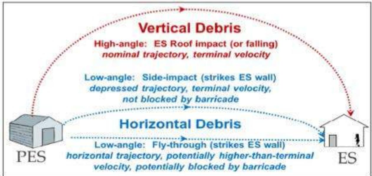
Fig.3. The design trajectories of primary fragments
