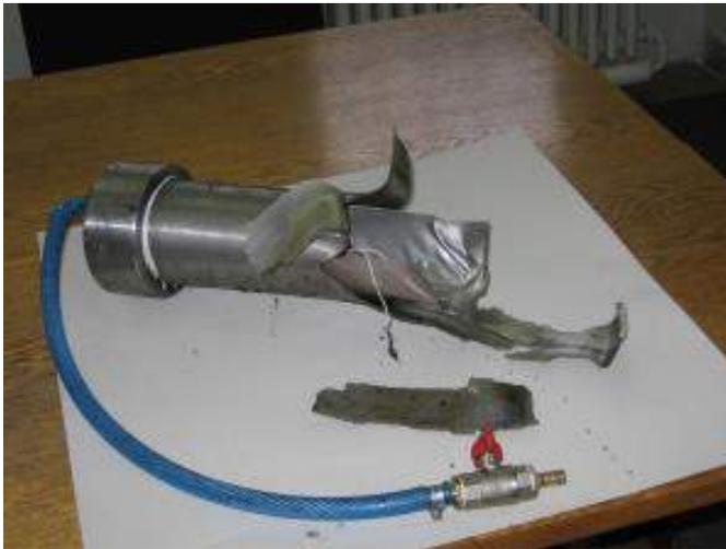
*Fig. 6.1.* State of cylinder no.1 after testing
