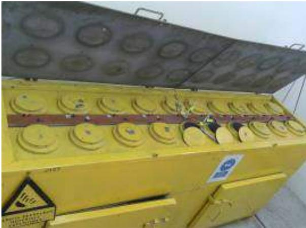
Fig. 3. Electric detonators prepared for testing
