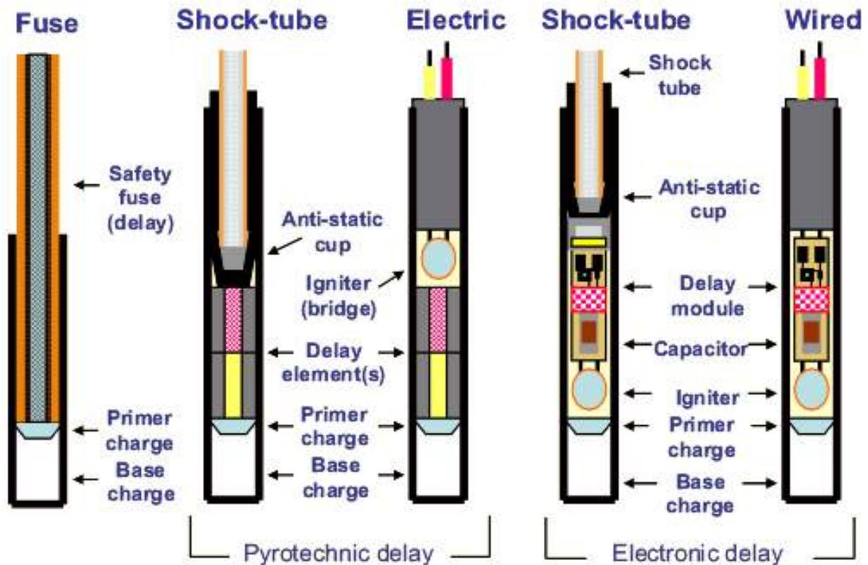
Fig.1. Constructive types of detonators for use in mining
