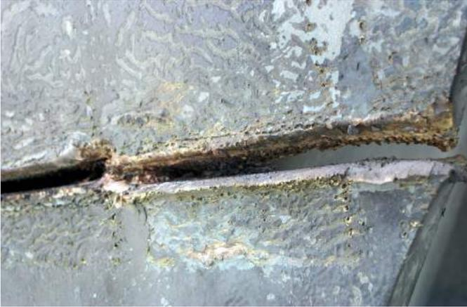
*Fig. 8: insufficient cut caused by splitting of shaped charges.*
