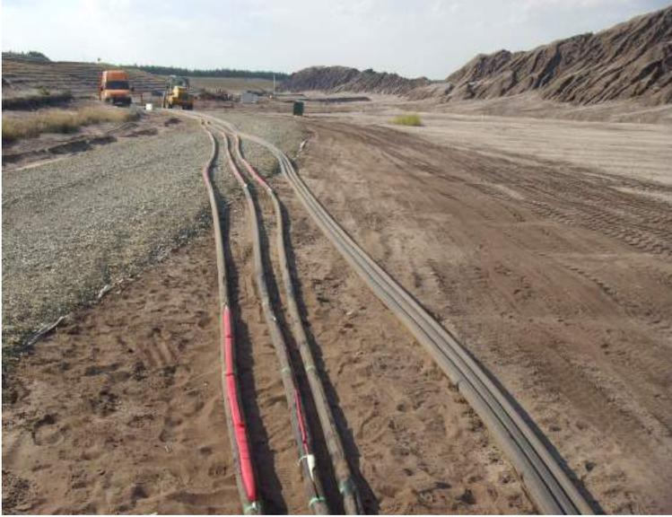
*Blasting Pipe with up to 14 decks/charges - realized
