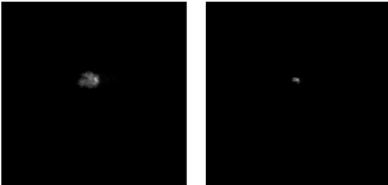
Fig. 4: Shot flames of a permitted detonator in firedamp, two time moments
