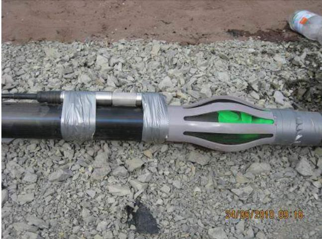
*Pore water pressure transducer prepared to use in horizontal drill holes (Test 1 und 2)*
