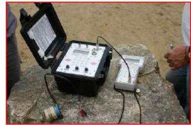
*Detonator, Connector Block, Blasting Machine and Logger (Austin Powder)*
