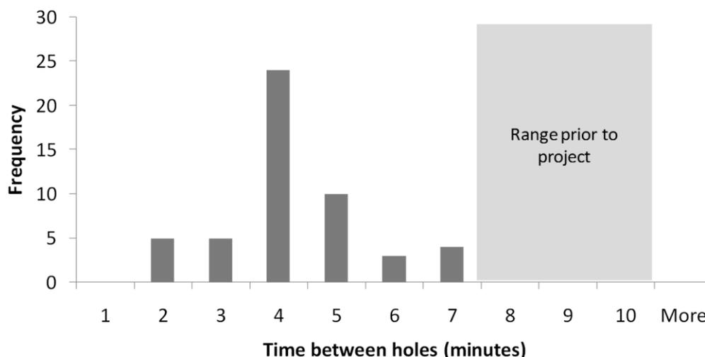
Figure 10. Improved charging cycle times due to automated blast loading (after Joseph, 2009)
