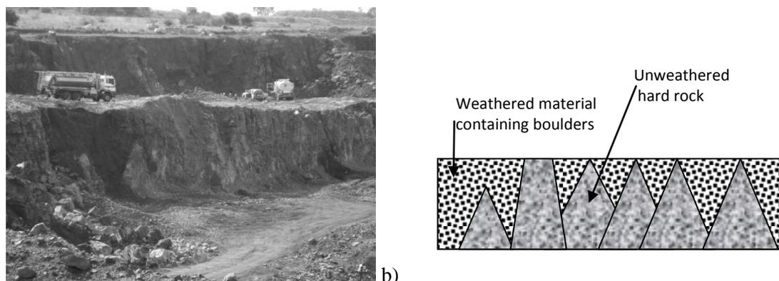
Figure 8. a) Photograph of top benches being charged and b) Schematic of rock cones interspersed with boulder material
